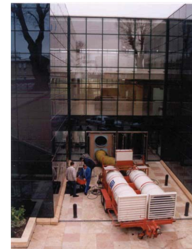
Banc grand volume Q_{\max} = 16\ 000\ \text{m}^3/\text{h}
